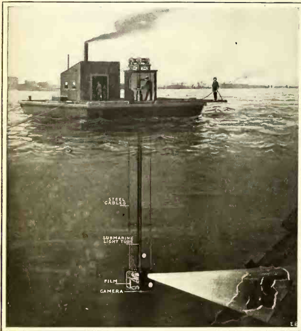
Proposed Scheme for Taking Submarine Motion Pictures by Means of Powerful Electric Searchlight Worked in Conjunction with the Camera From Above the Water's Surface.
