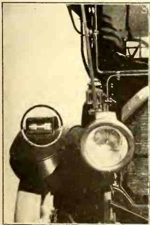
Effective Electric Auto Signal (in Circle) Tells Which Way Driver Intends to Turn.
