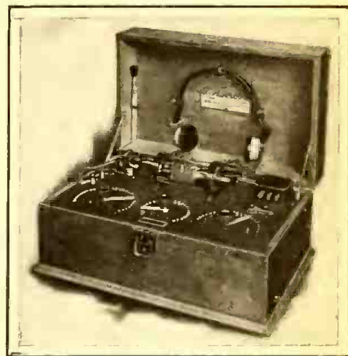
Newly-Developed Radio-Receiving Set Equipped With Crystallo Detector.
